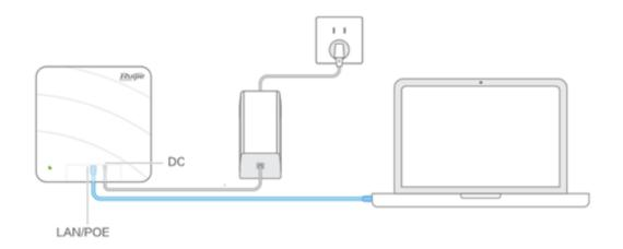
Note: Only part of the AP model supports DC power supply, there will be a corresponding DC interface identifier on the AP panel.
