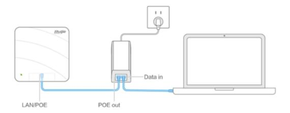
2. POE switch power supply connection diagram.
